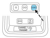
2. The display will change to CHANNEL "X" (1,2, or 3) TRAINING after 20 seconds. Without releasing the HomeLink® button, follow step 2 in the "Programming" section.
